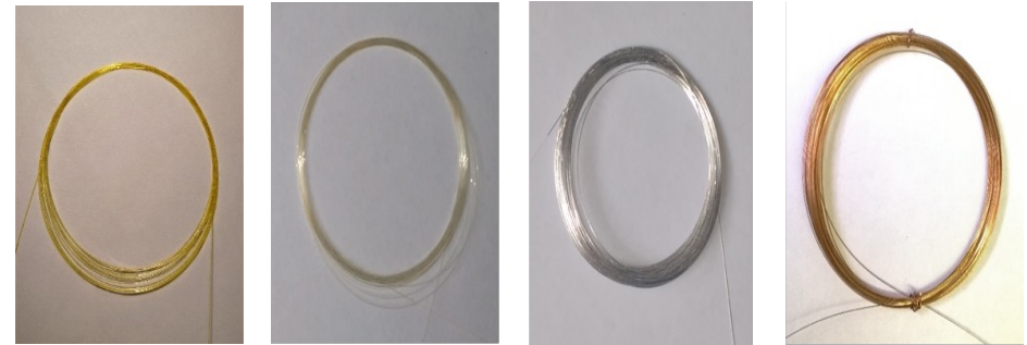
Photographs of optical fibers coated with FBG-based sensors designs polyimide, acrylate, aluminum, and copper (from left to right).
