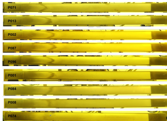
Microstructure evolution of irradiated KIMQI-FUTURE plates as a function of the burnup
